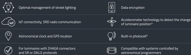
**ALZ 10x5** is an IoT module developed for remote monitoring and configuration of street lightning. The device gathers power metering and luminaire status data and transmits them via LoRa low power network or radio SRD technology to the acquisition server. The module is developed for universal 4-pin ZHAGA luminaires equipped with DALI interface and SR or DALI2 protocol.
