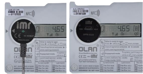
OLAN with applied Opto Head 01x1 (with USB connection) OLAN with applied Opto Head 02x3 (with Bluetooth BLE 4.1)
