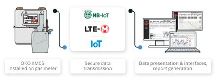
**OKO XM05** installed on gas meter takes pulses from the meter (appropriate adapter on request - see below) and can send the data over a wide variety of mobile networks to acquisition server. Subsequently, the data can be processed further to 3rd party data center.
