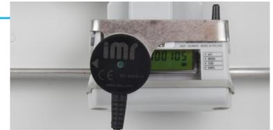
APULSE X3x5 with applied Opto Head 01x1 (with USB connection)
