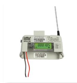
**NOTE** Cut the battery wires separately to avoid short circuit and uncontrolled discharge of the remaining battery power.
