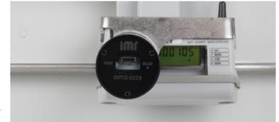
APULSE X3x5 with applied Opto Head 02x3 (with Bluetooth BLE 4.1)
